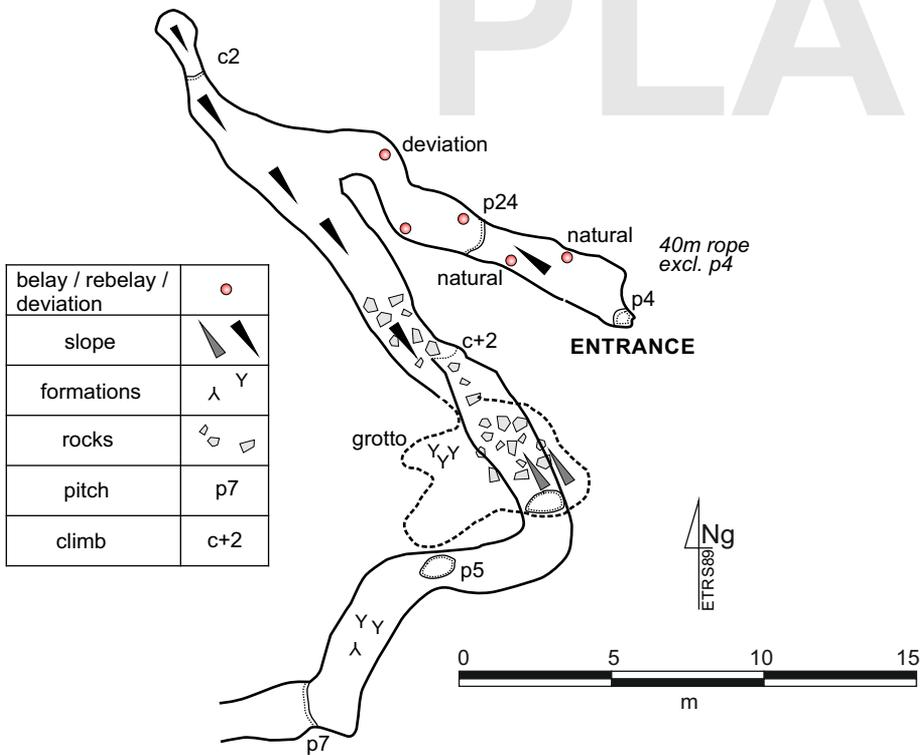
This cave survey is aligned to the ETRS89 grid which is 0.4 degrees to the west of True North.
