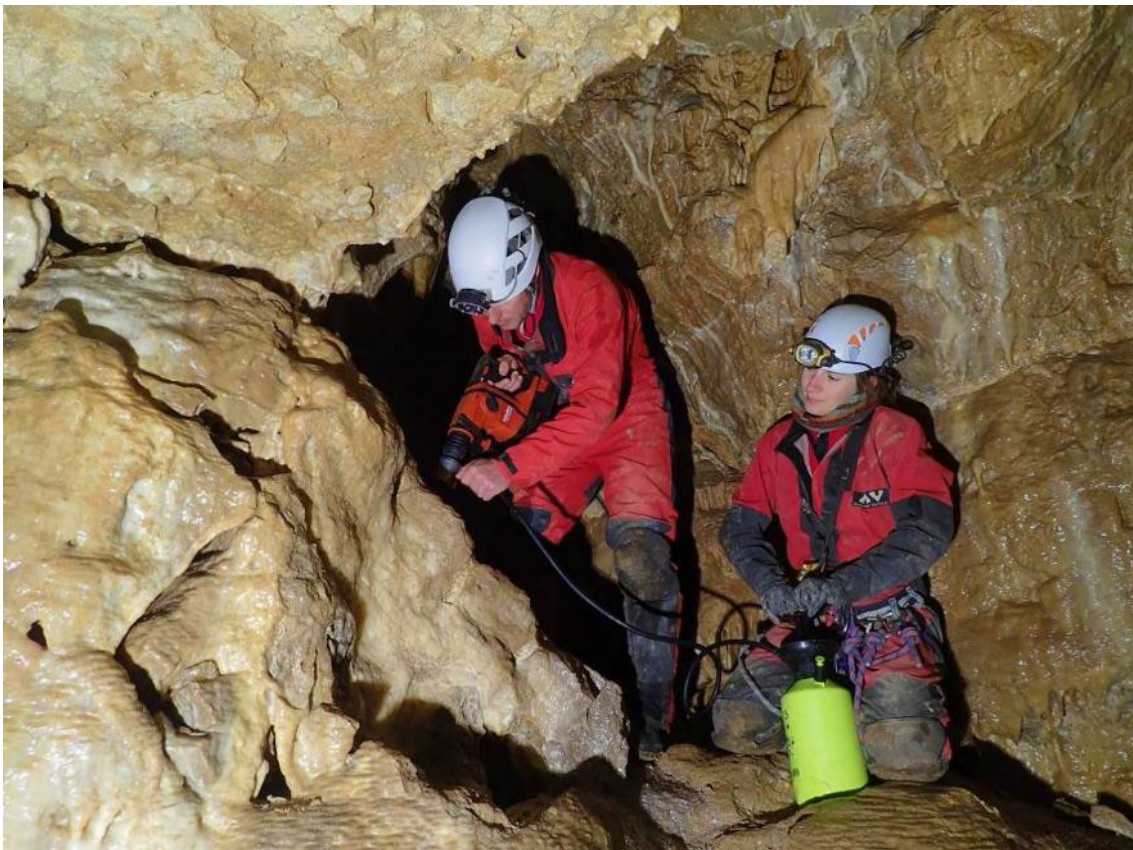
Coring a speleothem for palaeoclimate research, conducted under a permit at a Site of Special Scientific Interest in the UK. Photo by John Gunn.
