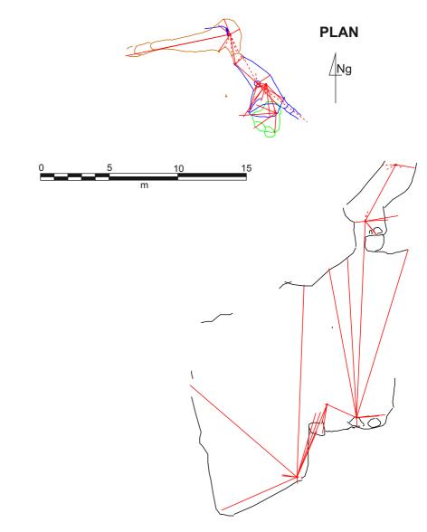
Drawings above are straight from the Pocket Topo software. The plan is to scale; the extended elevation may be.
